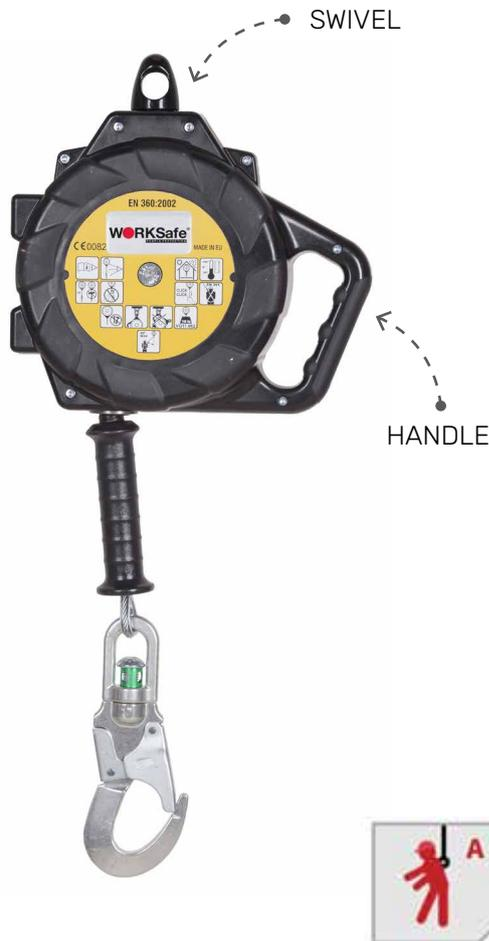
CR 250V is a self-locking device for vertical operation in a plastic casing with a pull-down steel rope and a swivel mounted in the casing. The device is designed for work requiring significant displacement in relation to the point of attachment. A shock absorber is not required. Available in 6m, 10m, 12m and 15m.
