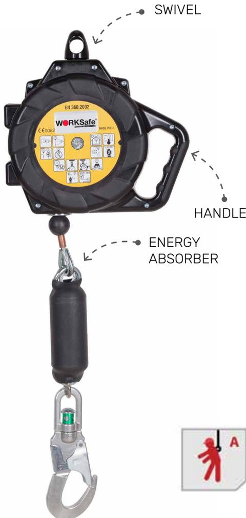
CR 250H + V self-locking device for vertical and horizontal operation in a plastic casing with a pull-down steel rope and a swivel mounted in the casing. The device has an additional shock-absorbing system located near the snap-hook. It is intended for work requiring considerable displacement in relation to the point of attachment. A safety shock absorber is not required. Also, the AZ 800 cable is not needed when working horizontally. Available in 6m, 8m and 11m.
