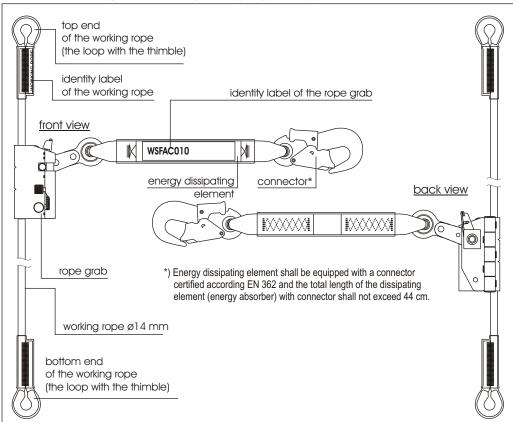
Using the WSFACO10 fall arrester in connection with fall arrest system must be compatible with use instructions of the fall arrest systems and obligatory standards:
